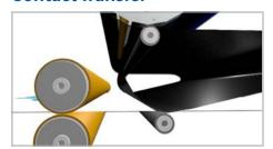
Transfers the image onto the media with precise alignment for accurate color registration through direct contact.
